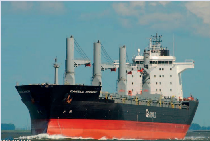
18. Canelo Arrow – bulk carrier type B 684 (48,041 DWT), 1996. Last ship built at Gdańsk Shipyard SA, 1990s. Photo: D. van Lear, public domain
