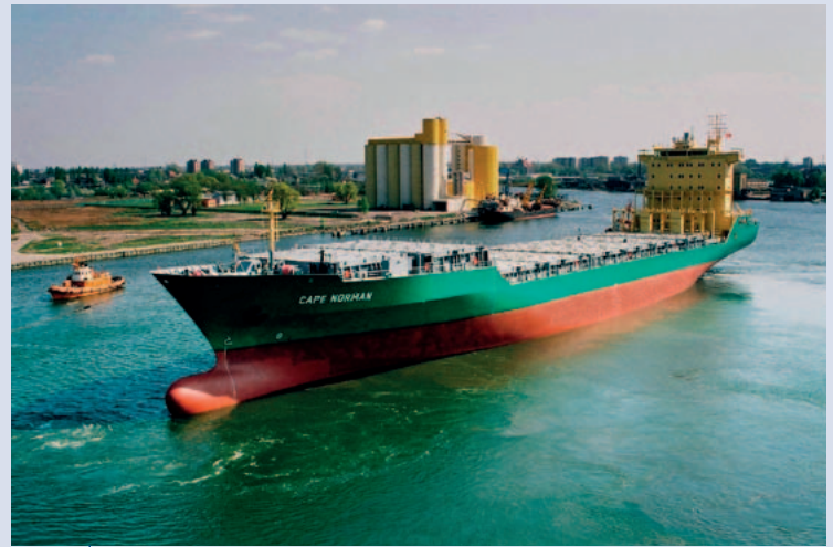
19. Cape Norman – type B 191 container ship (22,800 DWT), 1996. Photo: Z. Mirota, collection of the author
