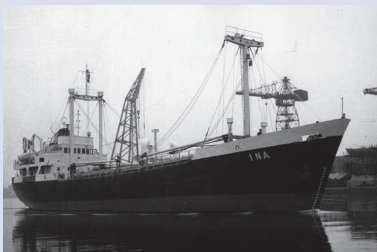
12. Ina – type B51 general cargo ship (690 DWT), 1958. The sixth ship in the first series of nine general cargo ships built at Gdańsk Shipyard between 1951 and 1959. Photo: Z. Mirota, collection of the author
