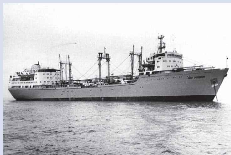
13. Pribałtika – type B 69 fish processing base (10,100 DWT), 1974. One of 68 fishing bases built at Gdańsk Shipyard, 66 were handed over to ship-owners from the USSR, 2 bases were built for Poland, 1970s. Photo: Z. Mirota, collection of the author
