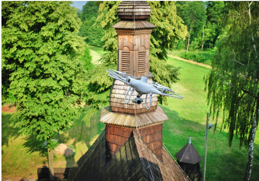
3 The drone is an indispensable tool for collecting photogrammetric data in inaccessible places. St Bartholomew's Church in Poręba Wielka (photo: K. Czajkowski)
