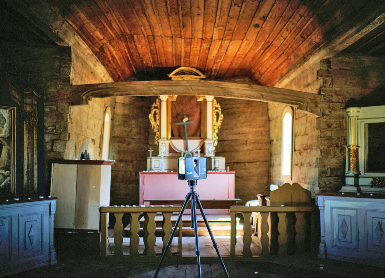
2 Laser scanning of the church of St Barbara in Solec nad Wisłą (photo: K. Czajkowski)
